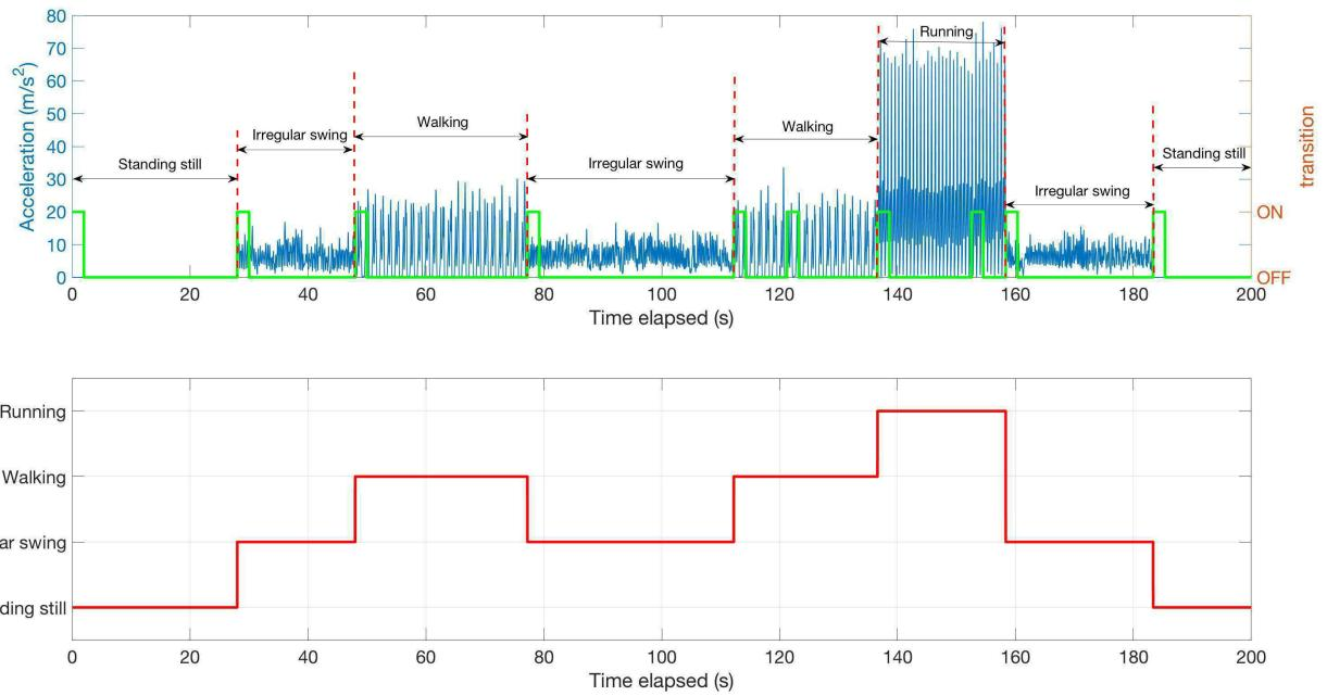
Fig. 5. The accelerations and identified behaviors
